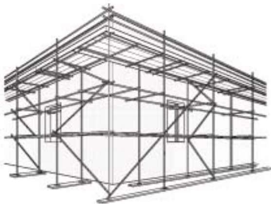
Typical independent tied scaffolding.
